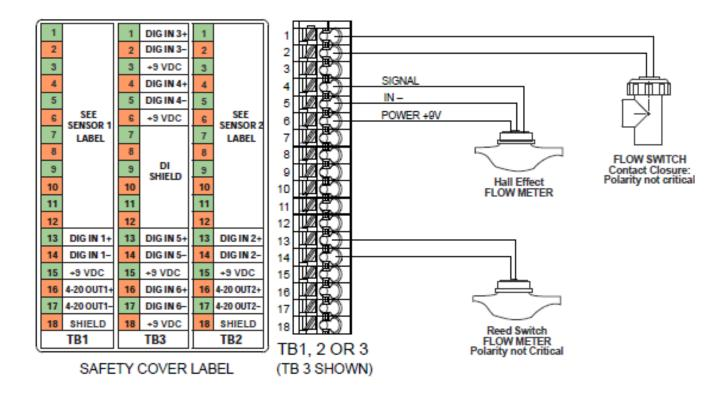
Figure 13 Digital Input Wiring
