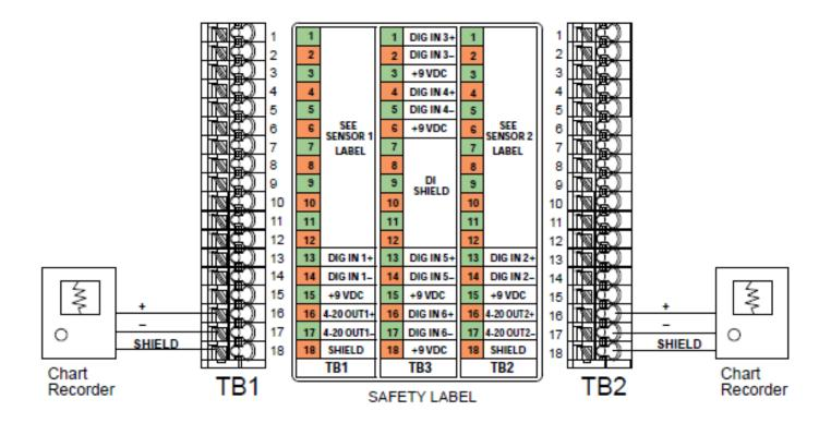
Figure 18 Analog Output Wiring
