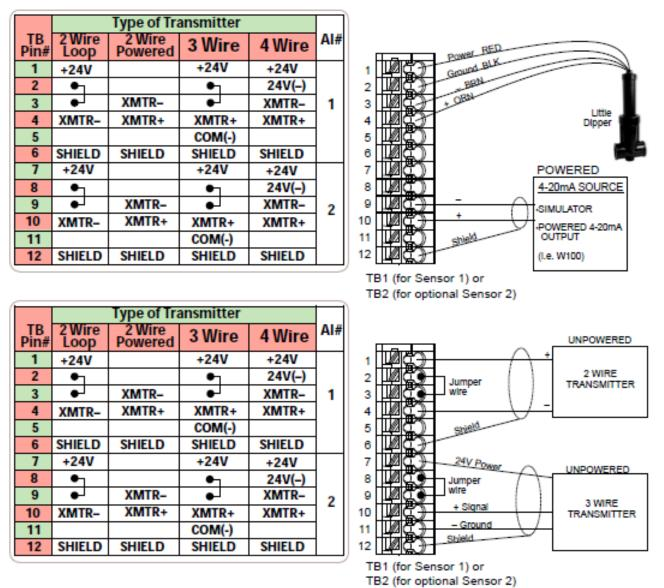
Figure 11 Dual 4-20mA Sensor Input Wiring
