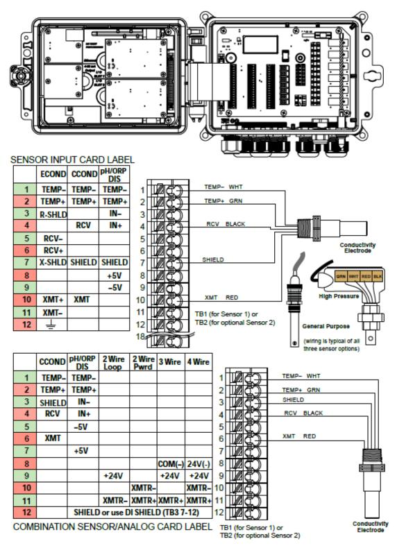
Figure 7 Contacting Conductivity Sensor Input Wiring
