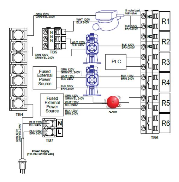
Figure 15 W610 AC Power & Relay Output Wiring
