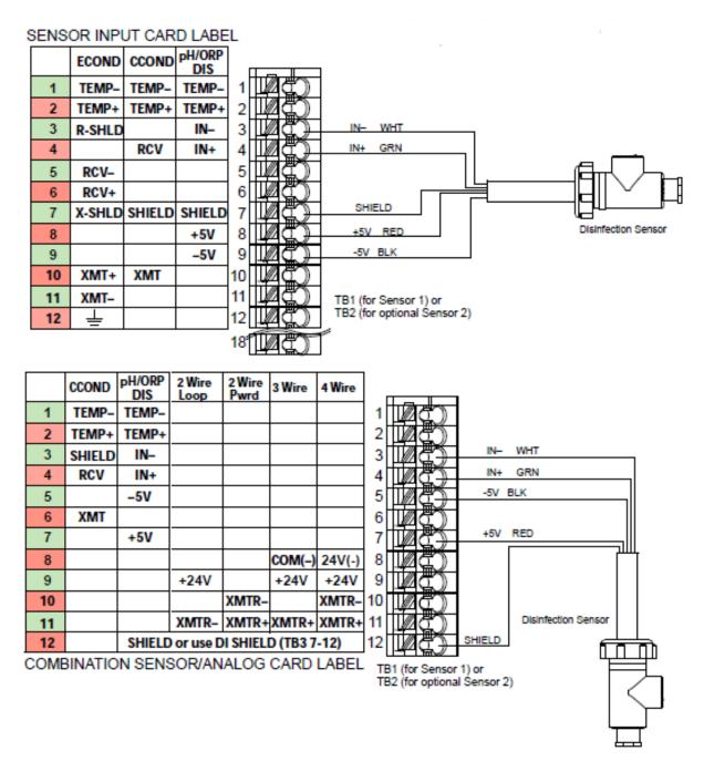
Figure 10 Disinfection Sensor Input Wiring
